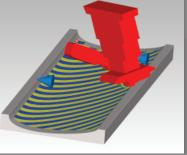
VCP reads CAD surfaces and ply boundary information and adds material to fill the plies according to user-specified manufacturing standards and requirements. Layup paths are then linked together to form specific layup sequences and output as NC programs for the automated layup machine.
